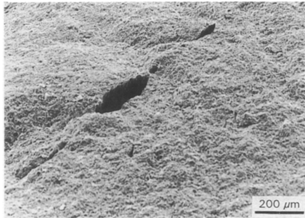
Figure 2 Scanning electron micrograph showing the linking together of fine pores to give failure in most test bars.
